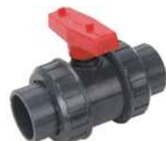
F71-Double Union Ball Valve Size: 1/2" TO 4" THREAD, SOCKET 1/2"-2": 235psi Max. 2- 1/2"-4": 150psi Max.
